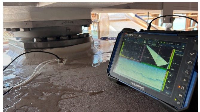
Phased array ultrasonic inspection
