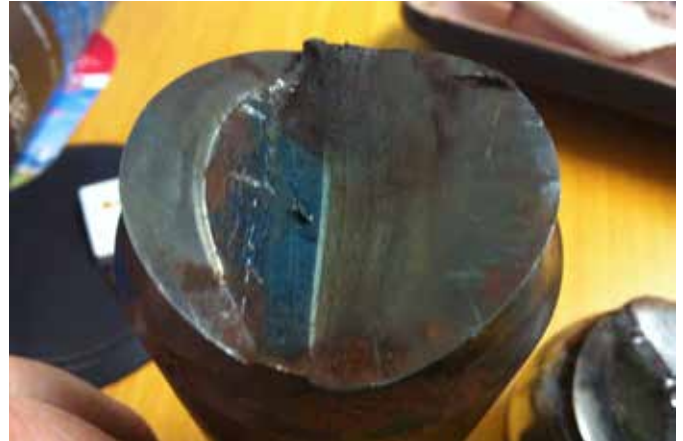
Fig. 8: Failed Ball Stud Showing Fatigue Beach Marks (up to ~70% cross sectional area) Before Brittle Fracture.
