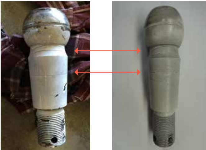
Fig. 9: Typical Cracked Studs (black circumferential lines are cracking)
