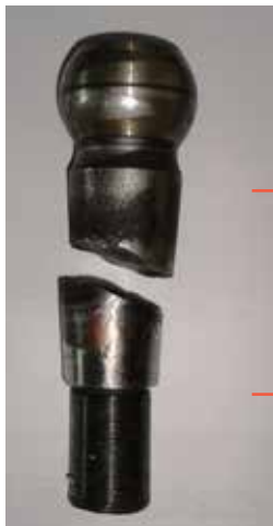
Fig. 3: Failed Ball Stud
