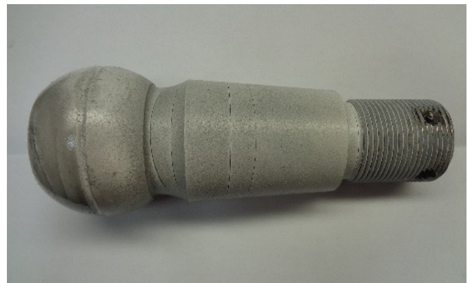
Fig. 6: Cotter Pin Holes (2 off) on a Cracked Cat 777 Ball Stud.
